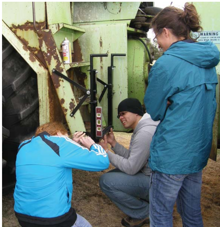
ABC Design Team members work on installing the spring-loaded step that they built and designed for their client.
