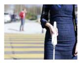
The <u>WeWALK Smart Cane</u> detects obstacles above chest level with an ultrasonic sensor and vibrates when these objects are near. It alerts users if there are low hanging trees, traffic signs, poles and other obstacles. It has mobile applications for both iOS and Android, and users can save favorite places and get turn-by-turn and clockwise navigation through the cane while the phone is in a pocket.
