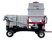
Workers with leg, arm, and back impairments can feed calves in hutches or pastured livestock with a <u>Feed and Water</u> <u>Transport Wagon</u>. Feed and water can be dispensed directly to troughs without lifting and carrying buckets by hand. The towable wagon consists of a feed hopper and a water tank (both polyester) mounted on a rubber-wheeled steel frame with hitching tongue. Custom-built according to users' needs, hopper sizes range from .8 to 2.8 tons and tank sizes from
