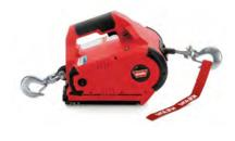
Although weighing only around 20 pounds, the remotecontrolled **Battery-Powered Portable Winch** can assist with many pulling/lifting tasks not only around the farmstead, but also out in the field and/or woodlot. Its brushless electric motor, which runs off a rechargeable lithium-ion battery, reportedly generates 1,000 to 2,200 pounds of pulling force at speeds of 5 to 25 feet per minute (depending on make/model).
