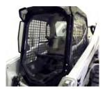
A <u>Skid-Steer Vinyl Cab Enclosure</u> is designed to protect from harsh working environment and the elements (e.g., cold, snow, wind, dust), which is especially important for persons with low energy, body temperature management issues, and/or arthritis. Features of this after-market product include: full 360-degree visibility, all-weather safety door, push-out rear window, reportedly simple attach/detach, and heavy-duty material used.
